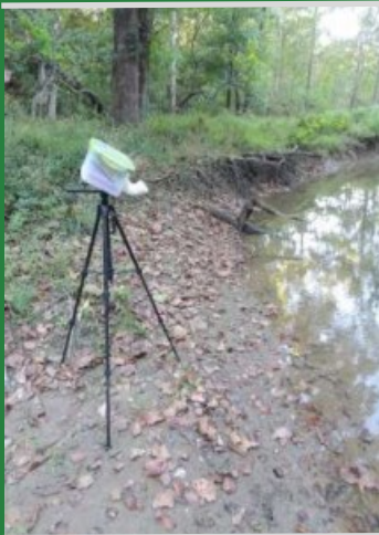
Photo, above: This device is an ultrasonic detector. It is able to record the ultrasonic sounds bats use for echolocation. These bat calls are later analyzed by looking at the frequency, shape, and other characteristics of the calls, the species of bat recorded can be determined.
